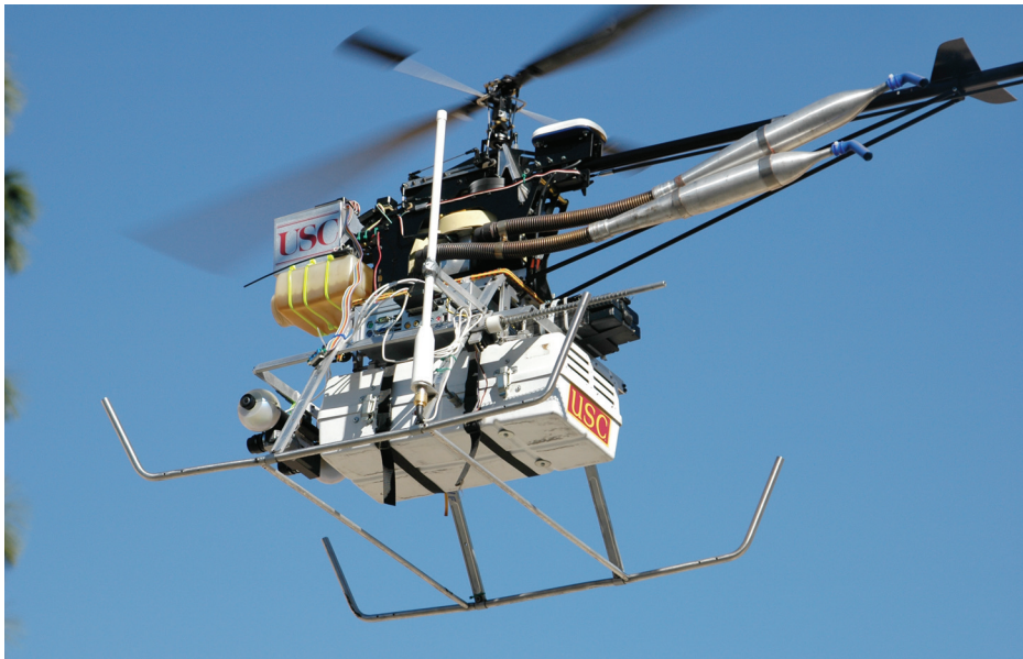
Figure 2 The AVATAR model remote control helicopter developed by USC's Autonomous Flying Vehicle Team utilizes a PC/104 stack for vision and another for flight control. It is capable of fully autonomous flight and includes flight-avoidance capabilities.
